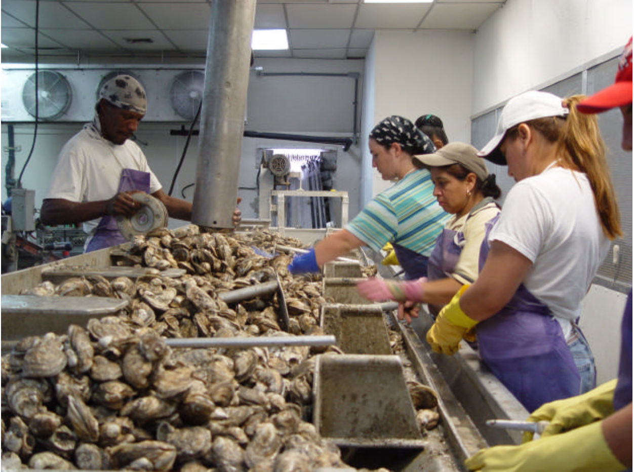
Figure 56. Shucked oysters being delivered to shucking table for meat separation from the shell.
