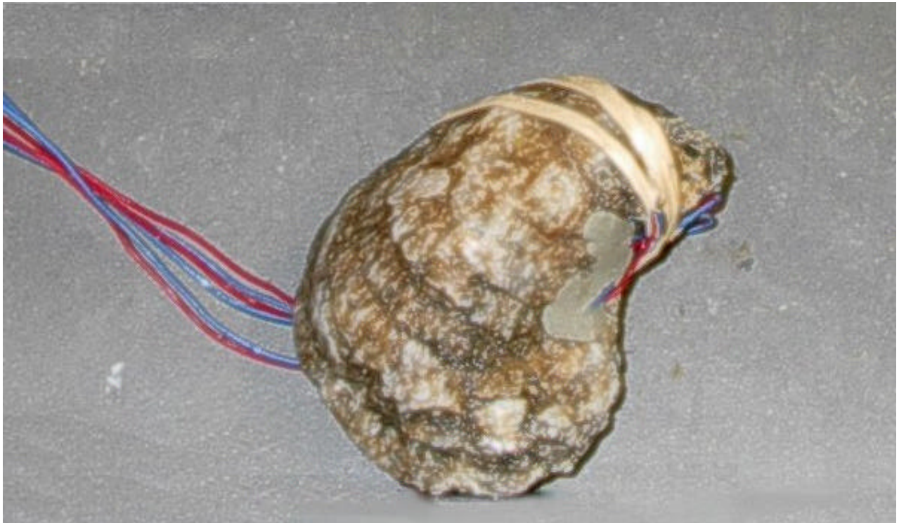
Figure 6. Instrumented oyster with clay plugs.
