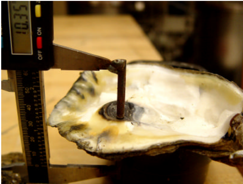
Figure 22. Digital calipers used to measure thickness of oyster shell at muscle scar.
