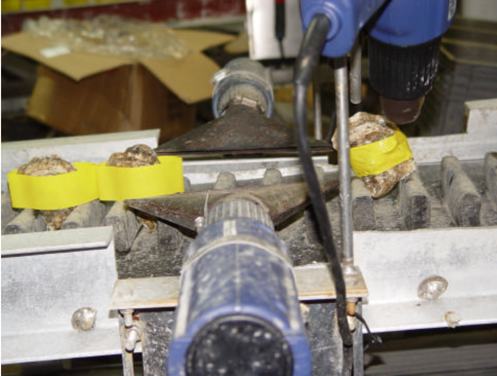
Figure 61. Heat guns used to shrink wrap heat-sensitive band around oysters.
