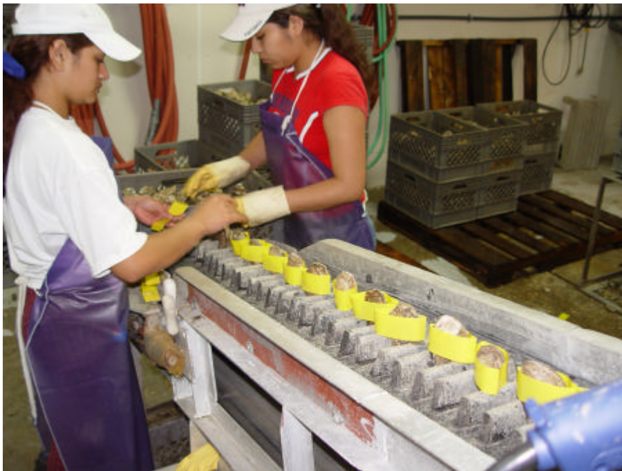
Figure 60. Banding of oysters prior to high pressure processing.
