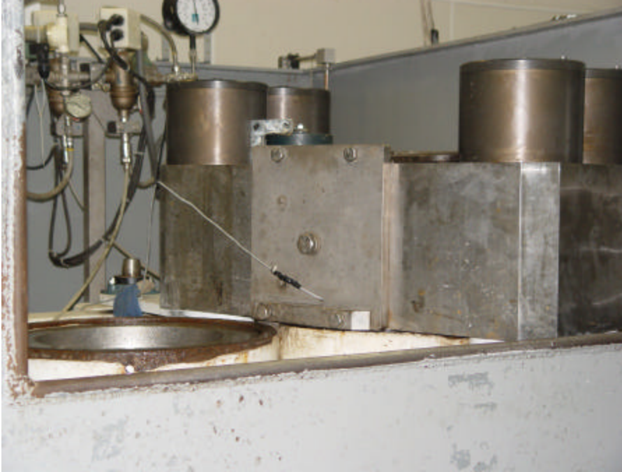
Figure 54. Closeup of high pressure vessel with two separate chambers for shucking oysters.
