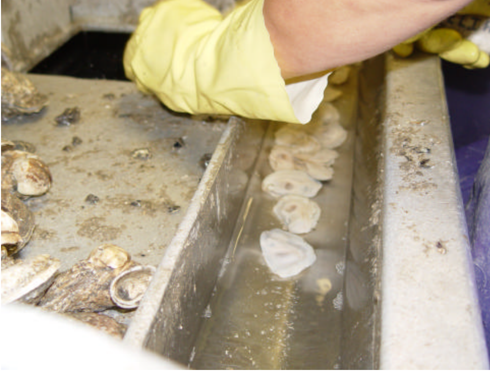
Figure 57. Shucked oysters being deposited into a water sluice for further washing.
