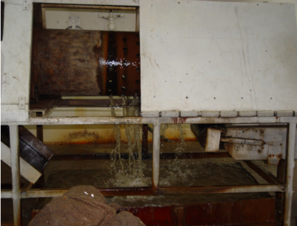
Figure 51. Rotating cylinder for cleaning and washing oysters prior to sorting and grading.
