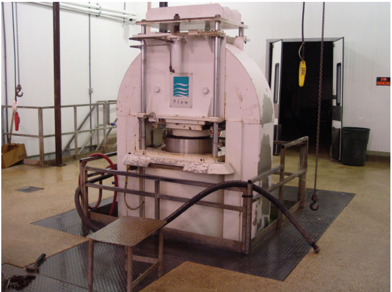
Figure 63. High pressure processing vessel at Joey Oyster.
