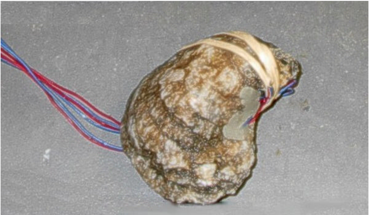
Figure 40. Instrumented oyster with clay plugs.
