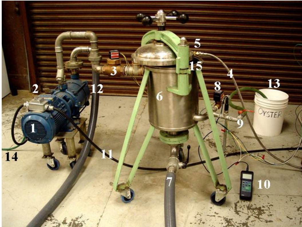
Figure 10. Automated oyster shucking system overview.
