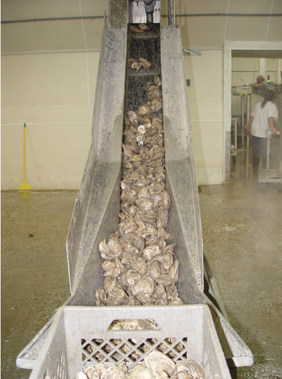
Figure 53. Oysters conveyed into cylindrical containers prior to pressurization.
