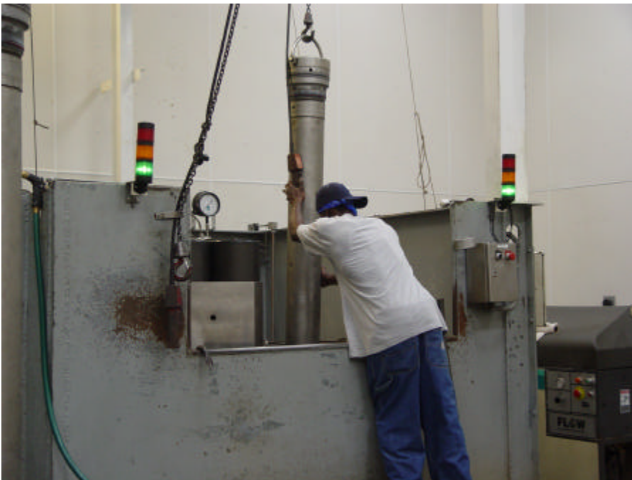
Figure 55. Cylinder of oysters being loaded into high pressure vessel at Motivait Seafood.
