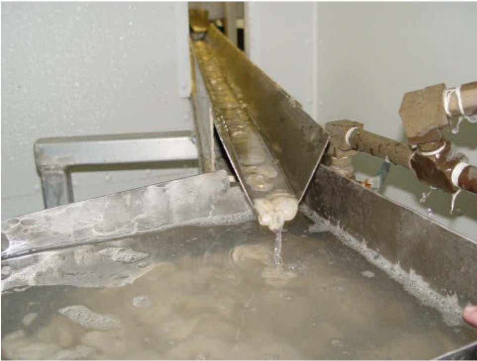
Figure 58. Shucked oysters traveling down sluice into cascading wash basin.
