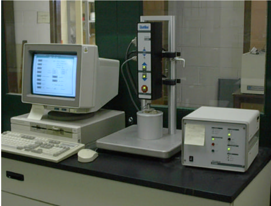
Figure 18. Vitrodyne hardware and setup for performing compressive resistance testing on oysters.
