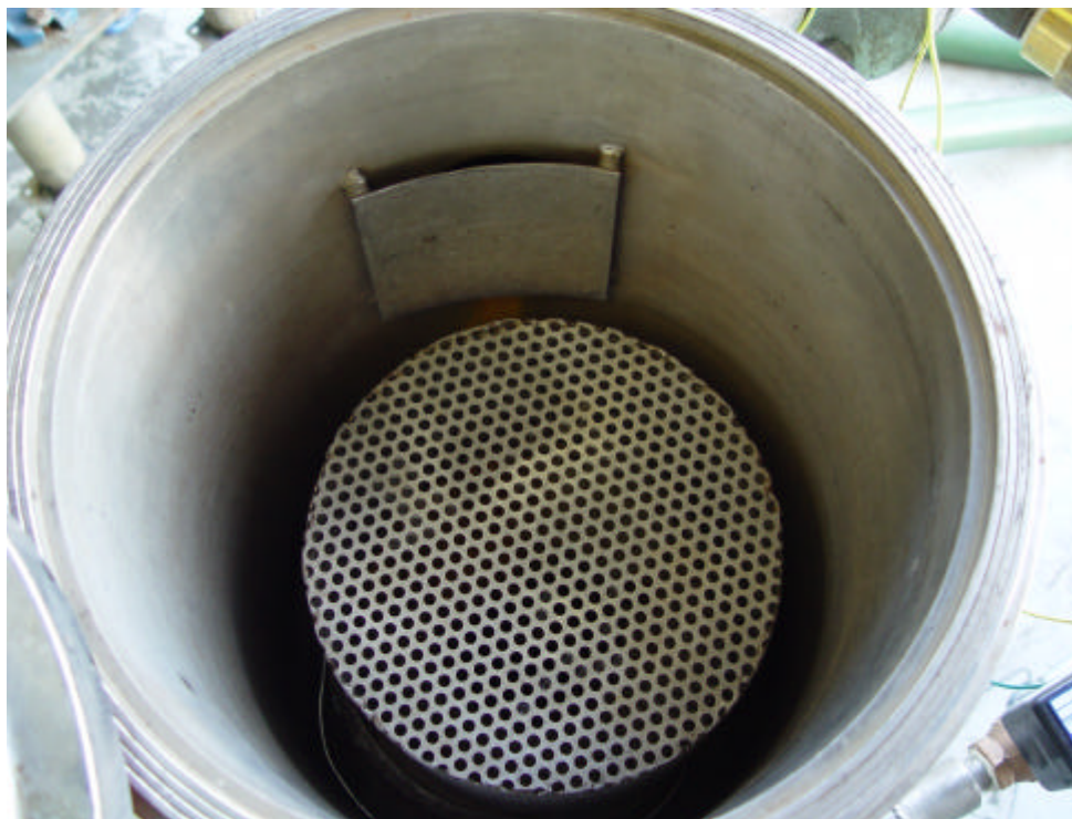
Figure 11. A view inside the steel retort.
