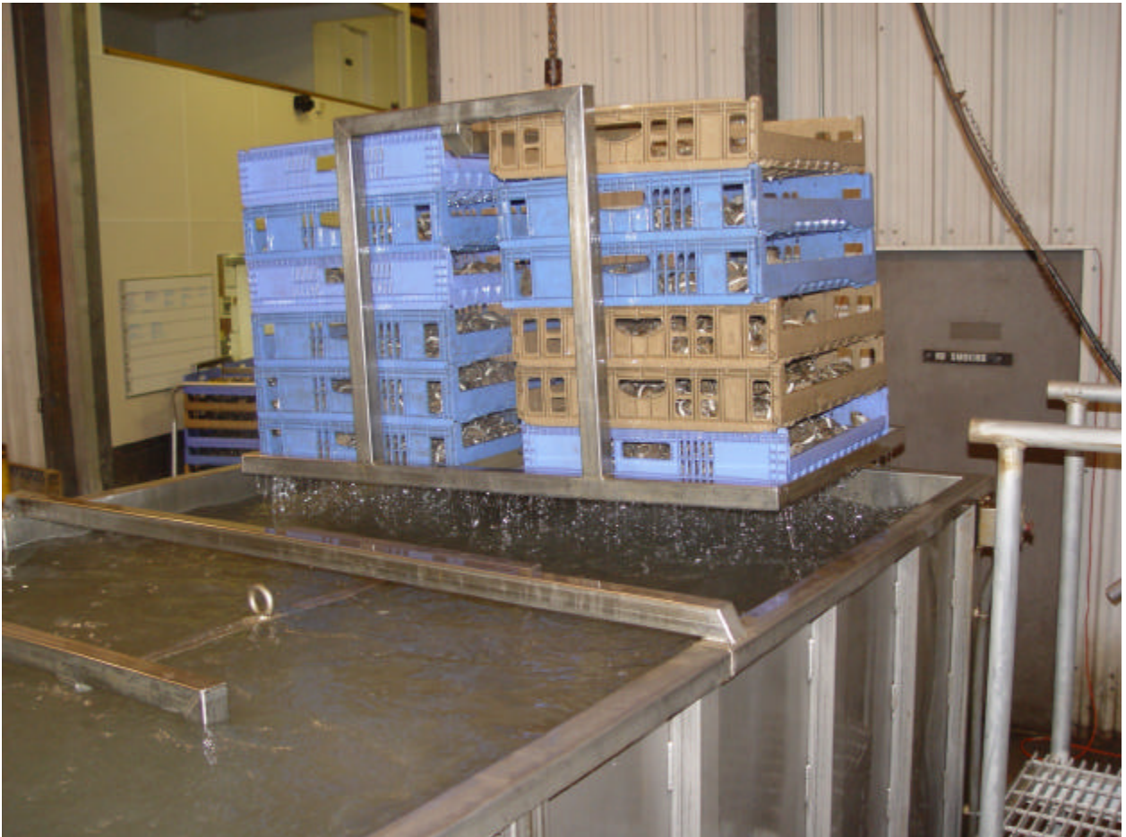
Figure 64. Banded oysters being immersed in warm water bath at Ameripure, Inc. to virtually eliminate Vibrio vulnificus .
